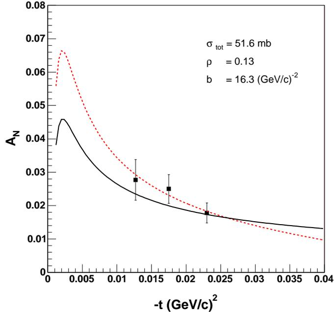
FIG. 4: The single spin analyzing power  $A_N$  for three  $t$  intervals. Vertical error bars show statistical errors. The solid curve corresponds to theoretical calculations without hadronic spin-flip and the dashed one represents the  $r_5$  fit.
