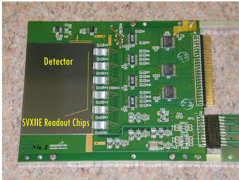
Fig. 4. An X-view detector board.
